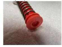
wipe out the barrel, spray the tip with silicon and then reassemble the syringe. With time and use, some of these tips, which Chemjet terms 'washers', would develop cracks as shown in the photo, and would no longer stay on the plunger. Chemjet sells a bag of 5 replacement washers for \$5, so I purchased an extra 10. But remember, by the time I was done with my project, each syringe had been used 70 or 80 times, so this certainly was not a quality issue.
